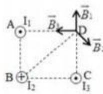
Chứng minh được:  $\vec{B}_D \not\sim \vec{B}_2$  nên  $B_D = |B_{13} - B_2| = \left| \frac{32}{3} \cdot 10^{-6} - \frac{32}{3\sqrt{2}} \cdot 10^{-6} \right| = \frac{16\sqrt{2}}{3} \cdot 10^{-6} = 7,54 \cdot 10^{-6} (\text{T})$ .
